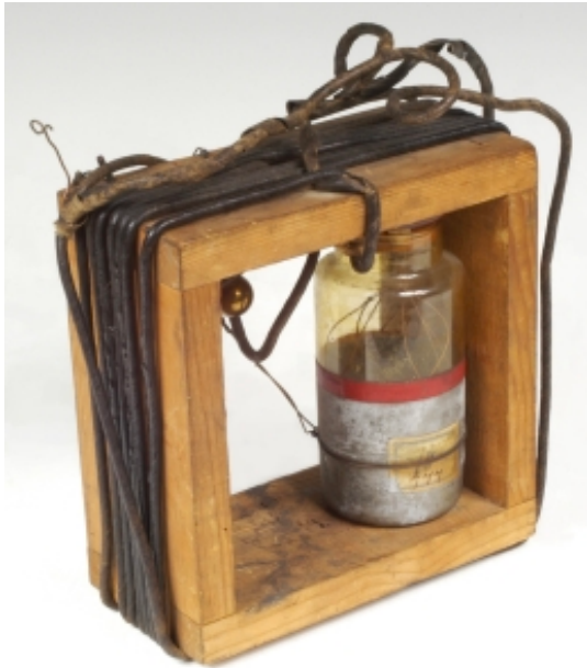
Marconi's first tuned transmitter, completed at the Haven Hotel, Poole 1899 - giving the ability to transmit waves at a specific frequency that a receiver can 'tune' in to, avoiding broadcasts interfering with each other.
