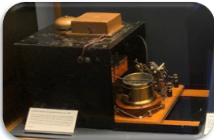
In 1896, Marconi used this Coherer Receiver to wow Victorian audiences with never-seen-before wireless technology – ringing a bell from anywhere in the room with no visible connection between the two. Marconi caused a sensation – and became a celebrity
